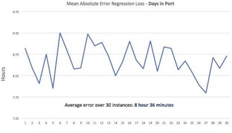
Separate instances of MAE outcomes using gradient boosting on 5-yr data using three (3) predictors
